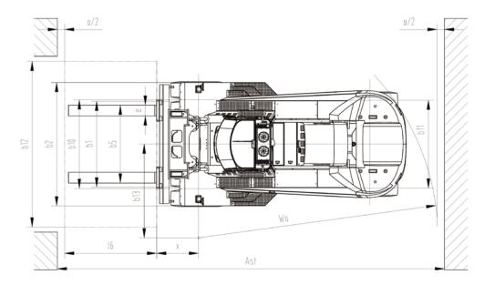
Ast=I6+Wa+x+a I6: load length a:Clearance(200mm)
